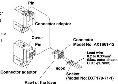
Note □ □ Do not pull the lead wire forcefully. Otherwise, connection failure and broken wire can result.
