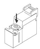
It is turned ON by pressing the manual override all the way in the direction indicated by the arrow (♣) and it is turned OFF by releasing it.
