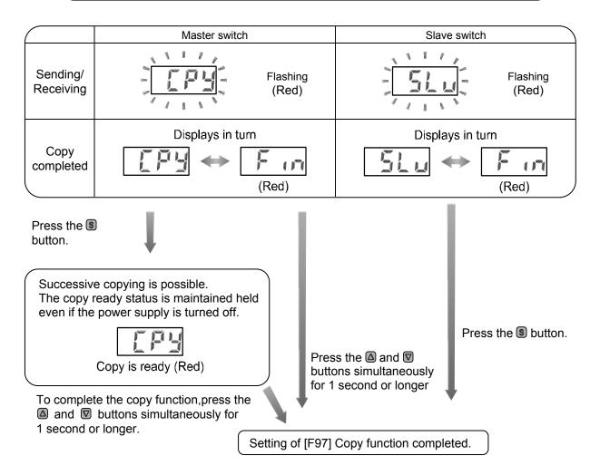
\*: If the copy to the slave switch is not completed, it is detected as a copying function sending/receiving error.
