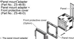
can be rotated through 90 degrees for mounting. Refer to the product catalog or SMC website (URL http://www.smcworld.com) for more information about panel cut-out and mounting hole dimensions.
