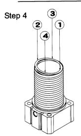
Apply ethanol to clean paper to wipe off dust on O-ring surface, and place the ring to O-ring groove. Press O-ring in numerical order in above drawing (press diagonally) to mount O-ring into the groove. which (Put on gloves generate no particle)
