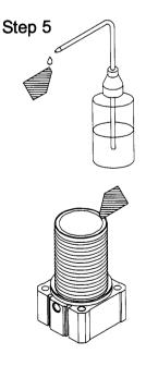
Apply ethanol to clean paper to wipe off dust on O-ring surface.
