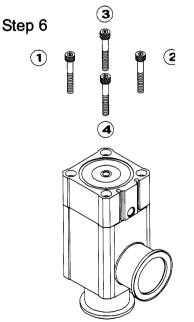
Supply 0.4Mpa of pressure to the port1(P)SUP to tighten bolts in numerical order in above drawing. First, hand tighten them evenly until just before O ring is squeezed. Then, tighten them altogether.
