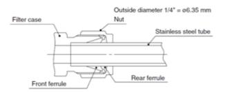
Regarding the TSJ fittings, after tightening the nut by hand, add another 1 1/4 to 1 1/2 turns with a wrench to seal the fitting. In case the fitting is re-installed after filter replacement, first tighten the nut by hand and add another 1/4 to 1/2 turns for sealing. Use the following parts as piping and fittings.
