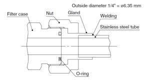
Weld the gland and piping when the fitting is used. At the time of welding, supply inert gas such as Nitrogen to the piping to prevent the formation of an oxide film. Also, remove the oxide film on the external surface through electrolytic polishing or acid cleaning.
