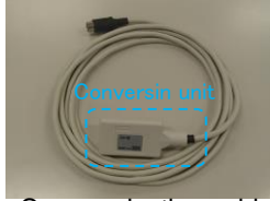
Communication cable & Conversion unit
