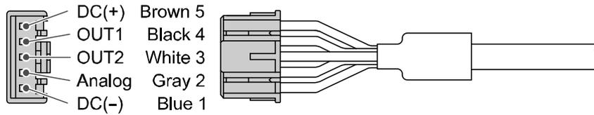
○ Internal circuit and wiring example
