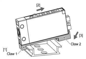
Engage claw 1 of the adapter on to the DIN rail as shown [1], apply force in direction [2], then press downward [3] until claw 2 clicks on to the DIN rail.
