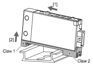
Move in the direction [1], and remove claw 1 in direction [2] as shown.
