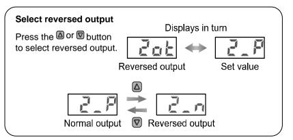
Press the S button to set. Move on to setting of pressure.
