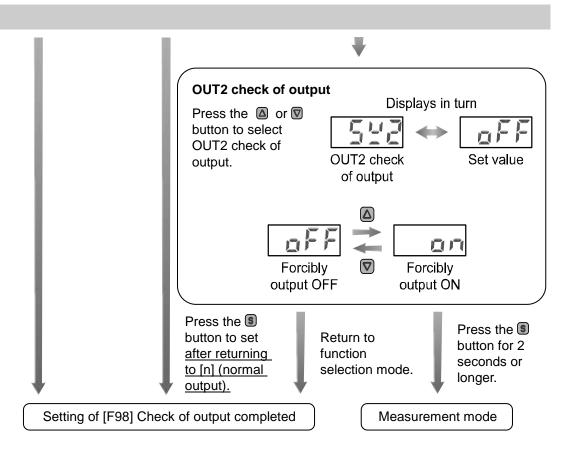
\*: If the \bigsilon button is pressed for 2 seconds or longer, the mode is returned to measurement mode regardless of the current mode.
