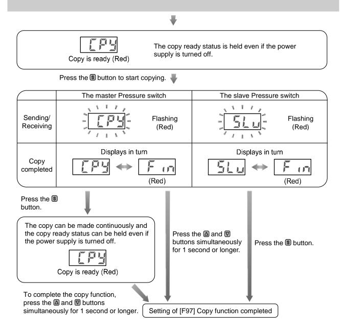
\*: If the copy to the slave Pressure switch is not completed, it is detected as a copy function sending/receiving error.
