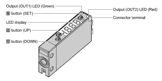
Output (OUT1) LED (Green): LED is ON when the switch output (OUT1) is ON.
