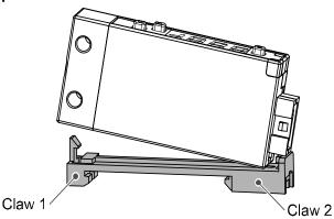
Engage the Pressure switch with claw 2 of the DIN rail adapter, then press down on to claw 1until it clicks.
