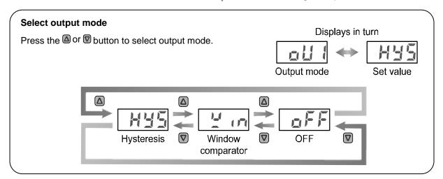
Press the S button to set. Move on to setting of reversed output.
