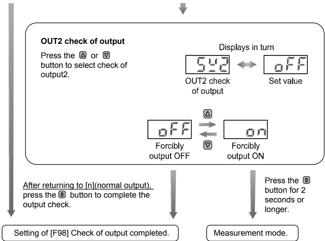
\*: Return to measurement mode from any point by pressing the  $\text{S}$  button for 2 seconds or longer.
