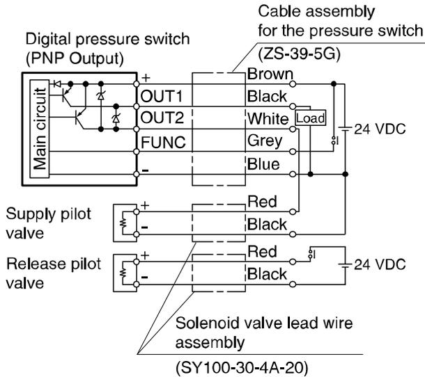
Integrated electrical entry for the pilot valves and the digital pressure switch
