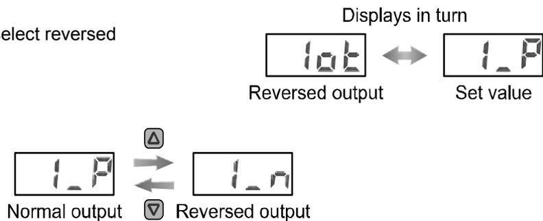
Press the **S** button to set. **↓** Move on to setting of pressure.
