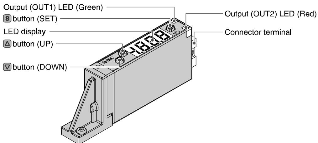
Output (OUT1) LED (green): LED is ON when the switch output (OUT1) is ON.
