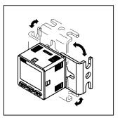
\*Bracket can be mounted on 4 sides.
