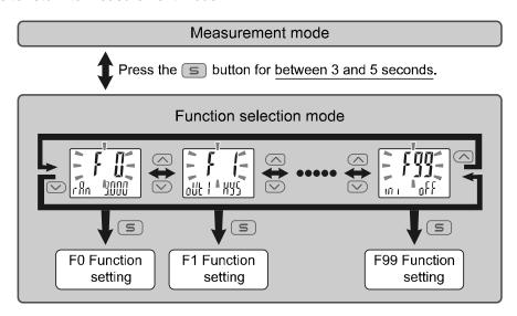
\*: Some products do not have all the functions. If no function is available or selected due to configuration of other functions, [- - -] is displayed on the sub display (right).
