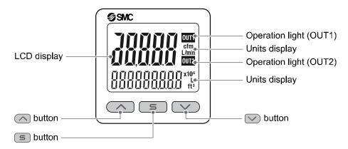
Operation light: Displays the switch operating condition.
