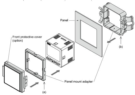
\*: The panel mount adapter can be rotated through 90 degrees for mounting.
