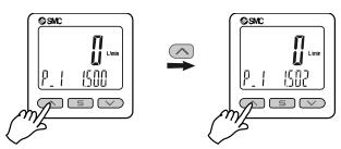
• Press the button once to reduce the value by one digit, press and hold to continuously reduce.
