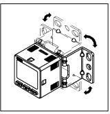
\*Bracket can be mounted on 4 sides.
