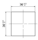
\*: Suitable for panel thickness of 1 to 3.2 mm.
