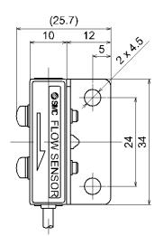
C \_\_\_\_\_ L-type bracket (Tapped) Mount on both sides
