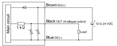
Analogue output: 1 to 5 V Output impedance: approx. 1 kΩ
