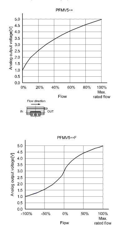
•Analogue output characteristics (Non-linear output)
