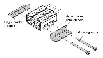
•Install the product (with bracket) using the M4 screws (4 pcs.).
