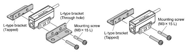
•Install the product (with bracket) using the M4 screws (2 pcs. or 4 pcs.).
