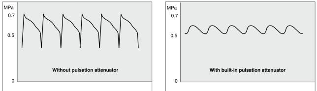
The process pump generates pulsation because it discharges a liquid using two diaphragms. The pulsation attenuator absorbs pressure when discharge pressure increases, and compensates the pressure when discharge pressure decreases. By this means pulsation is controlled.
