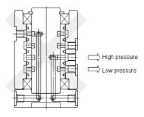
If neighbouring ports are used at different vacuum pressures, the vacuum pressure on the lower vacuum side will increase and hence it cannot be used.
