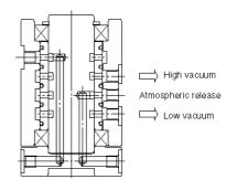
Using atmospheric release port
