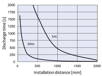
2) With Energy saving static neutralization cartridge For IZT40-112L, IZT41-112L
