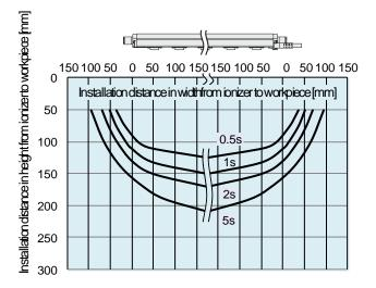
2) With High speed static neutralization cartridge, Supply pressure: 0.3 MPa For IZT40-□D, IZT41-□D
