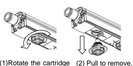
(1)Rotate the cartridge 90 degrees in the counter-clockwise direction.
