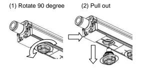
Removal procedure of emitter cartridge
