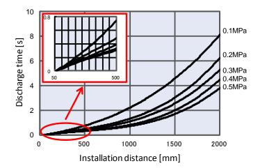
3) With Energy saving static neutralization cartridge With air purge, For IZT40-112L, IZT41-112L
