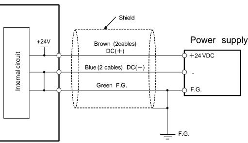
When the product is used in DC mode, make sure to ground the F.G. cable (green) and DC(-) cable (blue) of the input power supply with a resistance of 100 ohms or less. Without grounding the DC(-) cable, the ionizers and/or power supply may be damaged.
