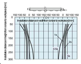
4) With Energy saving high-efficiency cartridge, Supply pressure: 0.3 MPa For IZT40-□V, IZT41-□V
