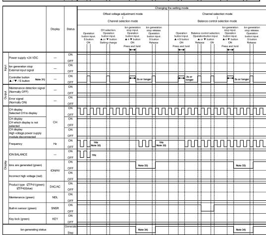
Note 31) Press the controller button once or for 2 seconds or longer to change/set of the setting mode and stop/release the ion generation. To release ion generation stop, press the S button once or turn the power off and on again.
