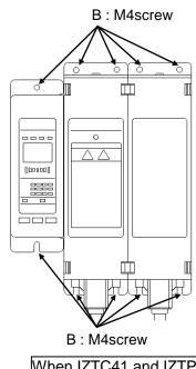
When IZTC41 and IZTP42 are directly connected.
