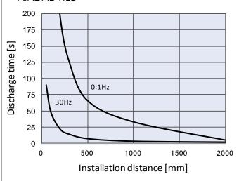
2) With Energy saving static neutralization cartridge For IZT42-112L
