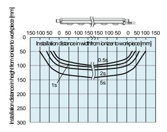
2) With High speed static neutralization cartridge, Supply pressure: 0.3 MPa For IZT42-□D
