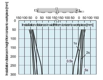
3) With Energy saving static neutralization cartridge, Supply pressure: 0.3 MPa For IZT40-□L, IZT41-□L
