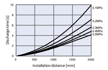
3) With Energy saving static neutralization cartridge With air purge, For IZT42-112L
