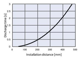
2) With High speed static neutralization cartridge With air purge, For IZT40-112D, IZT41-112D
