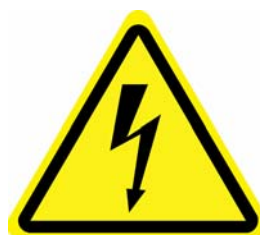
Fig. 1-2 Warning Label for High Voltage
