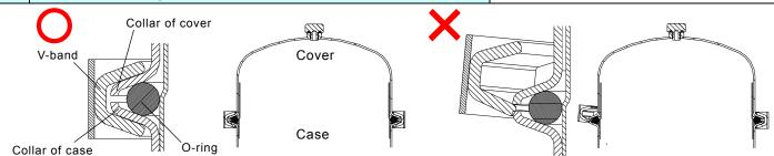
Fig. (a) Correct mounting of V-band
