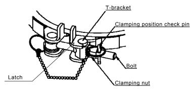
Fig. (c) V band tightening
