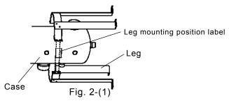
(2) Close the legs, and mount the hexagon head bolts and nuts, which are delivered together with the product, onto the bolt mounting holes on the legs and tighten them at 12.5 Nm.
