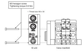
Remove the M3 hexagon screws from the SI unit and release the SI unit from the valve manifold.
