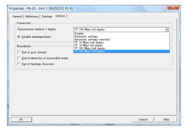
•Configuration of the EX260-SPN to enable the FSU function Select the EX260-SPN icon from the dialogue of the HW configuration window. Double click the Slot X1 Interface and in the "General" window check "Prioritized startup".
