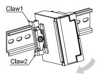
2. Tighten the mounting bracket screw, and fix the SI unit to the DIN rail. (Tightening torque: 0.6 Nm)
