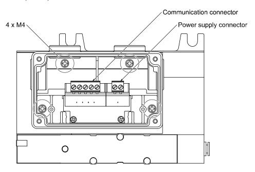
3. Remove the manifold wiring from the SI unit.
