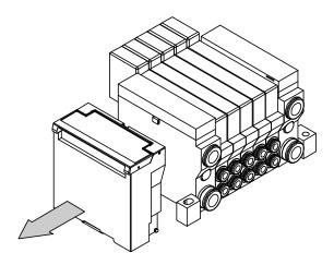
•Precautions when opening the cover When opening the cover, hold both sides of the cover.
