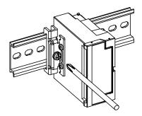
2. Remove the SI unit by unhooking claw 2 then claw 1.
