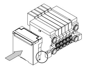
2. Confirm that the SI unit and manifold are securely locked together, and slide the SI unit downwards.
