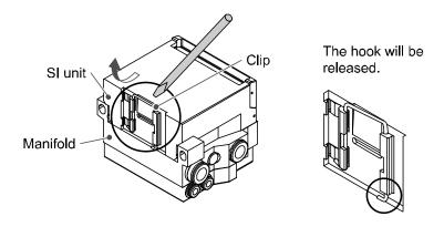
2. Slide the SI unit upwards with the clip pulled.
