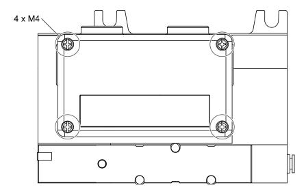
2. Disconnect the wiring from the SI unit, and remove the SI unit from the manifold. Disconnect the wiring to the SI unit.
