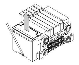
3. This releases the lock. Pull the SI unit slowly and remove from the manifold.
