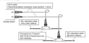
The M12 cable, AS-i standard cable and connector for T-branch are not supplied by
