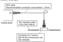
The M12 cable, AS-i standard cable and connector for T-branch are not supplied by
