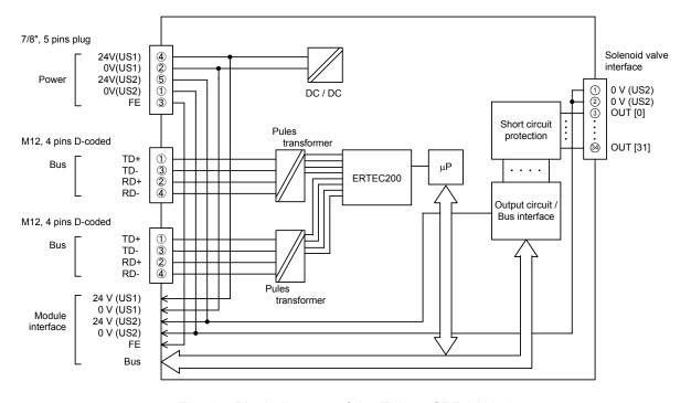
Fig. 9-5 Block diagram of the EX245-SPR1-X171
