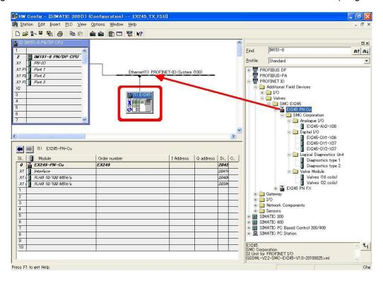
Fig. 7-7 Add EX245 onto a PROFINET network
