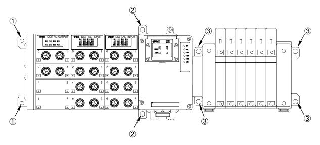
Fig. 6-1 Required screws
