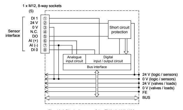
Fig. 13-3 Block diagram of the EX245-AX2-X38
