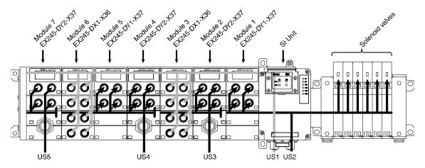
Fig. 4-1 Diagram of power supply concept (example)
