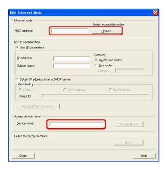
Fig. 7-6 Specify or find a unit and assign its "Device name"
