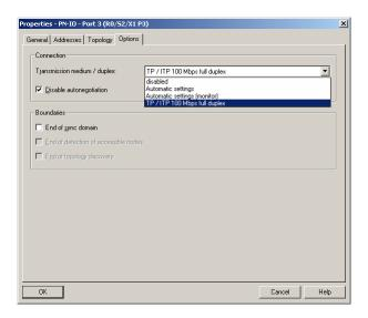
Fig. 7-12 Configure the PROFINET port of the controller for FSU
