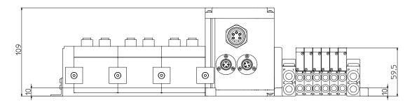
Fig. 14-4 Dimensions of the SV1000 manifold
