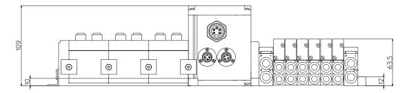
Fig. 14-5 Dimensions of the SV2000 manifold
