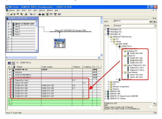
Fig. 7-9 Configure EX245 valve manifold
