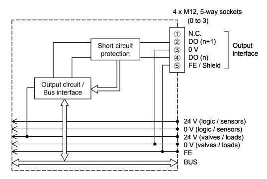
Fig. 11-3 Block diagram of the EX245-DY1-X37
