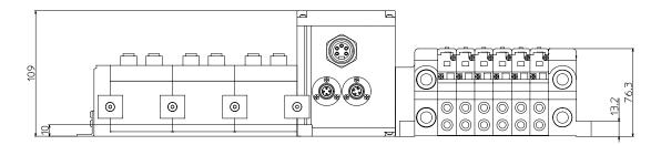
Fig. 14-2 Dimensions of the VQC2000 manifold
