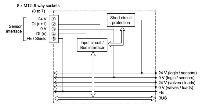
Fig. 10-3 Block diagram of the EX245-DX1-X36
