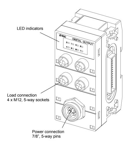
Fig. 12-1 Allocation of parts on the EX245-DY2-X37
