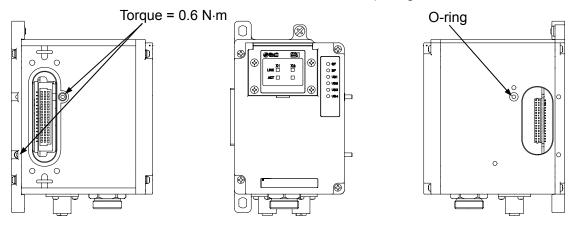
Fig. 6-2 Valve manifold connection
