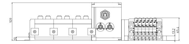
Fig. 14-1 Dimensions of the VQC1000 manifold
