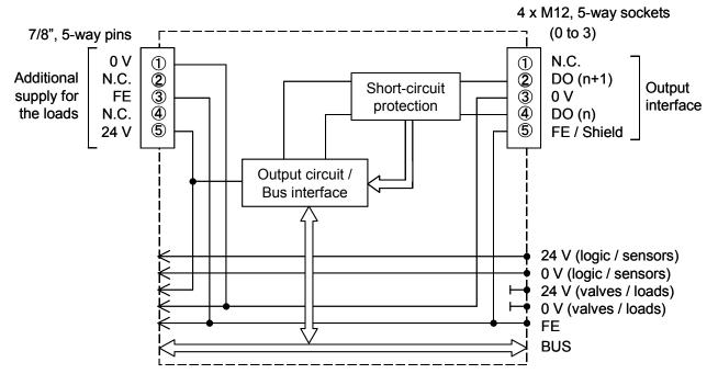
Fig. 12-3 Block diagram of the EX245-DY2-X37
