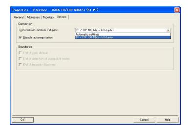
Fig. 7-14 Configure PROFINET port of the EX245-SPR1-X171 for FSU
