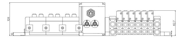
Fig. 14-6 Dimensions of the SV3000 manifold
