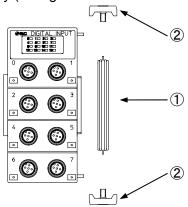
Fig. 6-3 Module connection
