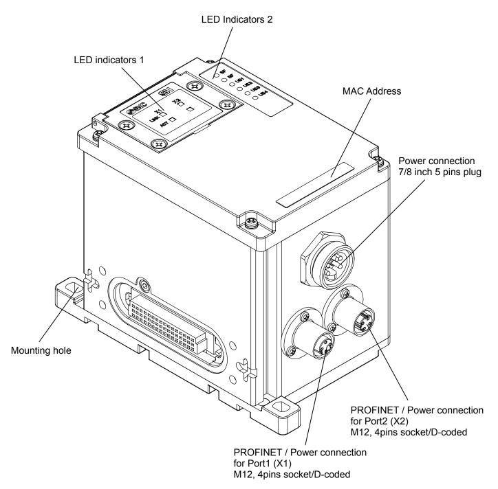
Fig. 9-1 Allocation of parts on the EX245-SPR1-X171
