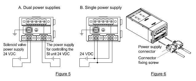
\*: Communication connector FG and FG terminal are connected inside the SI unit. Ground one of the terminals with the ground resistance of 100  $\Omega$  or less.
