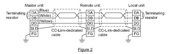
(3)The terminating resistance to be connected to the CC-Link network depends on the type of cables used. (Refer to the table below. Figure 3)
