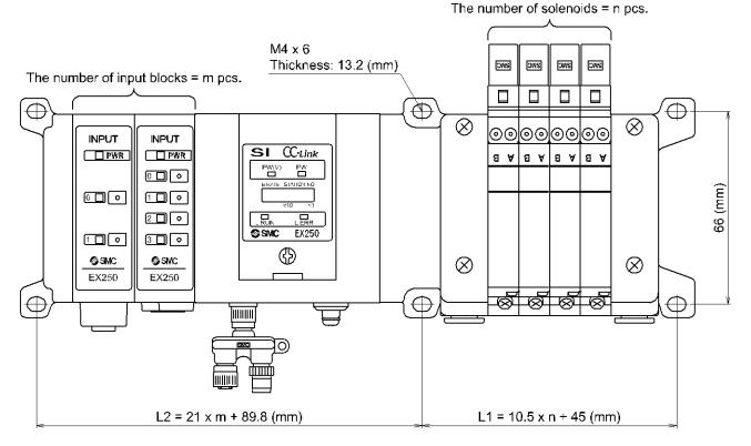
For example, the table below shows the size when manifold of VQC1000 series connected. Please refer to an individual catalog for the size when other manifolds are connected.
