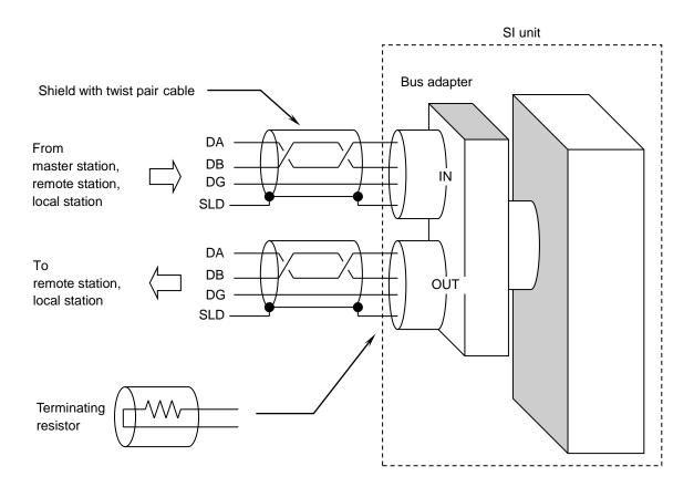
Shield (SLD) is connected to the ground terminal (FE) inside of the SI unit.
