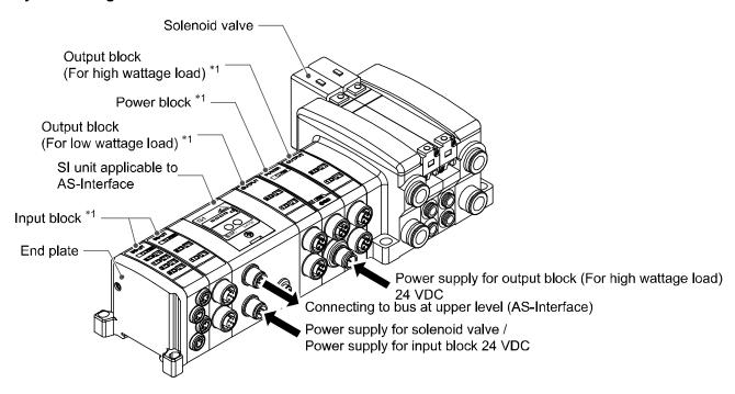
This system connects input/output devices to AS-Interface with reduced wiring. AS-Interface communicates with the input/output devices via the SI unit.
