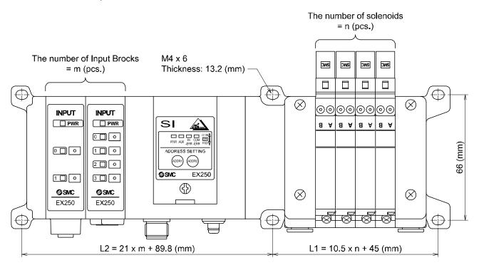
Dimensions when VQC2000 series solenoid valve manifold is connected are shown in the table below for reference.
